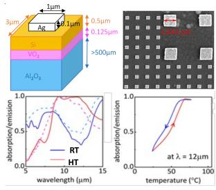
Schematic of a VO2 based passive thermal control metasurface (top-left). SEM image (top right) of the fabricated passive thermal control metasurface on VO2 film. Measured emissivity response of the fabricated sample (bottom-left) at room temperature (RT) and at high temperature (HT). Measured hysteresis at wavelength 12µm (bottom-right).
