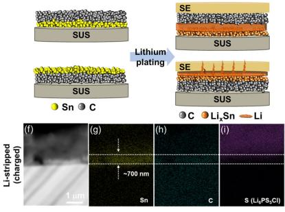
The all-solid-state battery showed uniform Li plating/stripping due to the novel Sn/C buffer layer deposited onto a stainless-steel current collector.
