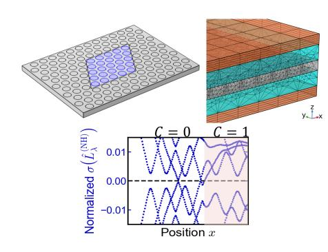
Schematic of a topological photonic slab heterostructure (top left) and its associated finite element mesh (top right). The system's local Chern marker identifies that the heterostructure's center is topological (bottom).
