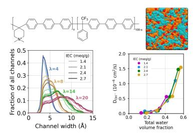
Simulations of a piperidinium-functionalized polymer (upper left) nanophase-separate into water (blue) and polymeric channels (orange) (upper right). The size of the water channels depends on water content  $\lambda$  but less on the IEC (lower left). The hydroxide ion diffusion constant depends on water volume fraction (lower right).
