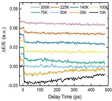
The transient change in terahertz transmission as a function of temperature (T) due to the photoinduced carriers. The fast decrease is due to thermalization of the spin and lattice systems; the slow recovery is due to electron-hole recombination which is >10 nanoseconds at high T and occurs on a sub-nanosecond timescale in the magnetic phase (low T).
