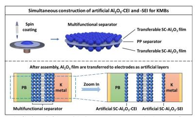
A thin film (10  $\mu$ m) of alumina (Al<sub>2</sub>O<sub>3</sub>) nanopowder is spin-coated on both sides of commercial polypropene separators, then transferred onto both anode and cathode surfaces during cell assembly. This creates both artificial solid-electrolyte interphase (SEI) and cathode electrolyte interface (CEI) that enhance electrochemical kinetics of potassium metal batteries (KMBs).
