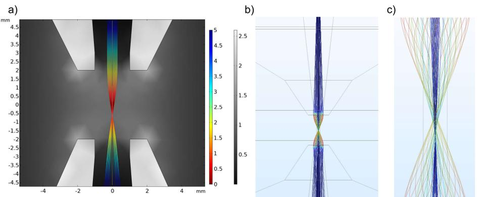
Figure 5: Charged particle tracing simulations in (a) 2D and (b & c) 3D. In both cases, the crossover point is visible, with the spiralling trajectories visible for the 3D case. Rainbow colourmap in (a) represents vertical distance from the sample midplane for clarity, while black & white colourmap represents the magnetic flux density. Colourmap in (b&c) represents radial distance from central axis.
