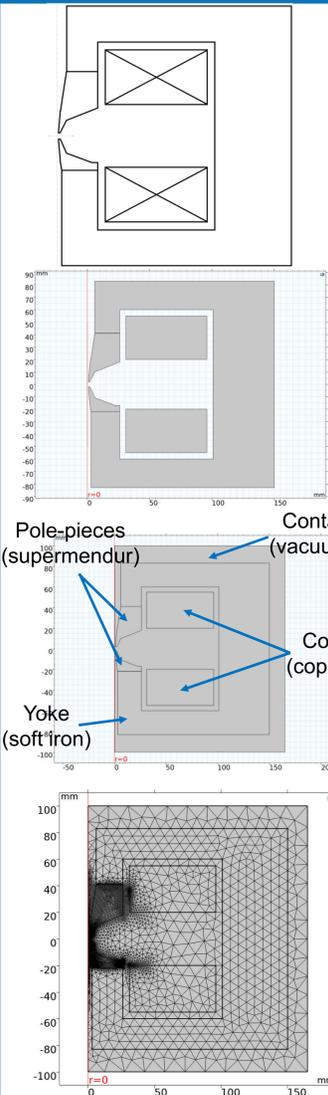
Though 3D models can be simulated, the OL can be approximated as being cylindrically symmetrical and a 2D simulation can be performed, saving computation time. Figure 2 details the steps followed;
