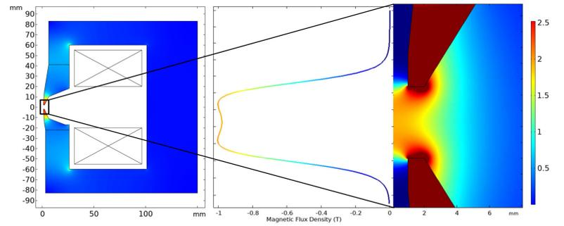
Figure 3: (Left) The simulated magnetic flux density in the objective lens of a TEM. (Middle) Magnetic flux density along the optical axis. (Right) Zoom to show the concentration of flux density at the pole-piece tips. The vacuum sample region has also been included. Colourmap indicates magnitude of flux.
