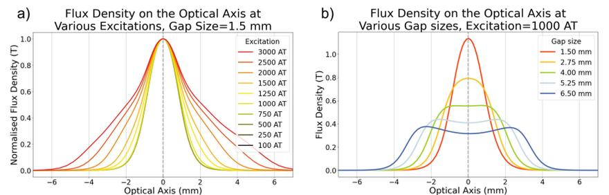
Figure 4: Simulated flux curves along the optical axis for various levels of lens excitations (a), and gap sizes (b). This lens saturates just below 1000 AT, where the FWHM of the curve begins to increase. The thin lens approximation is not suitable for larger gap sizes, where significant aberrations are introduced.
