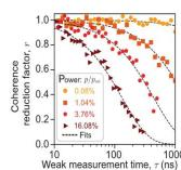
Measurement of the ratio of remaining to initial coherence,  $r=|\hat{\rho}'_{\uparrow\downarrow}|/|\hat{\rho}_{\uparrow\downarrow}|$  where  $|\hat{\rho}^{(r)}_{\uparrow\downarrow}|$  is the off-diagonal density matrix element before (after) measurement.
