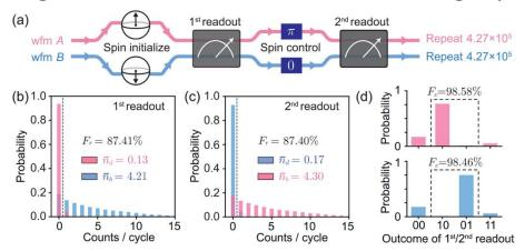
Single-shot readout of a single electron spin. (a) Readout sequence repeated for  $4.27 \times 10^5$  cycles. (b,c) Count distribution of  $1^{st}$  and  $2^{nd}$  readouts showing single-shot readout fidelity of 87.4%. (d) Conditional fidelity of a 2-shot readout sequence of 98.5%.
