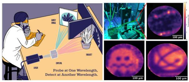
Left: Cartoon illustrating principles of quantum ghost imaging. Top Middle: Picture of sorghum plant in quantum ghost microscope. Top Right: Quantum ghost microscope transmission image of live sorghum leaf. Bright spots are rows of stomata.
