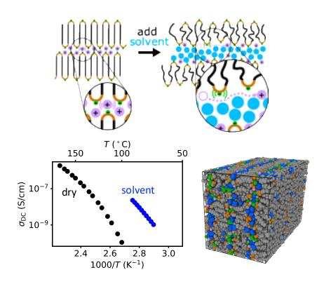
An ionic multiblock polymer that forms layers (top left, Li<sup>+</sup> in purple) can be swollen with solvent (blue, top right) which enables higher Li<sup>+</sup> conductivity (blue, bottom left). Simulations reveal the Li transport mechanism (bottom right).
